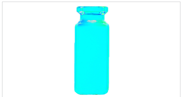
Example 2: Residual mechanical stress check in Glass Bottle
