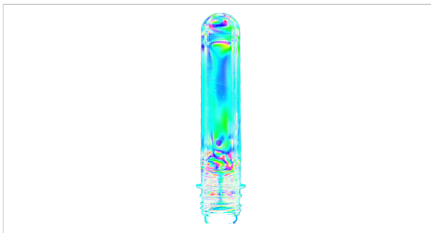
Example 1: Residual mechanical stress check in Plastic Preform
